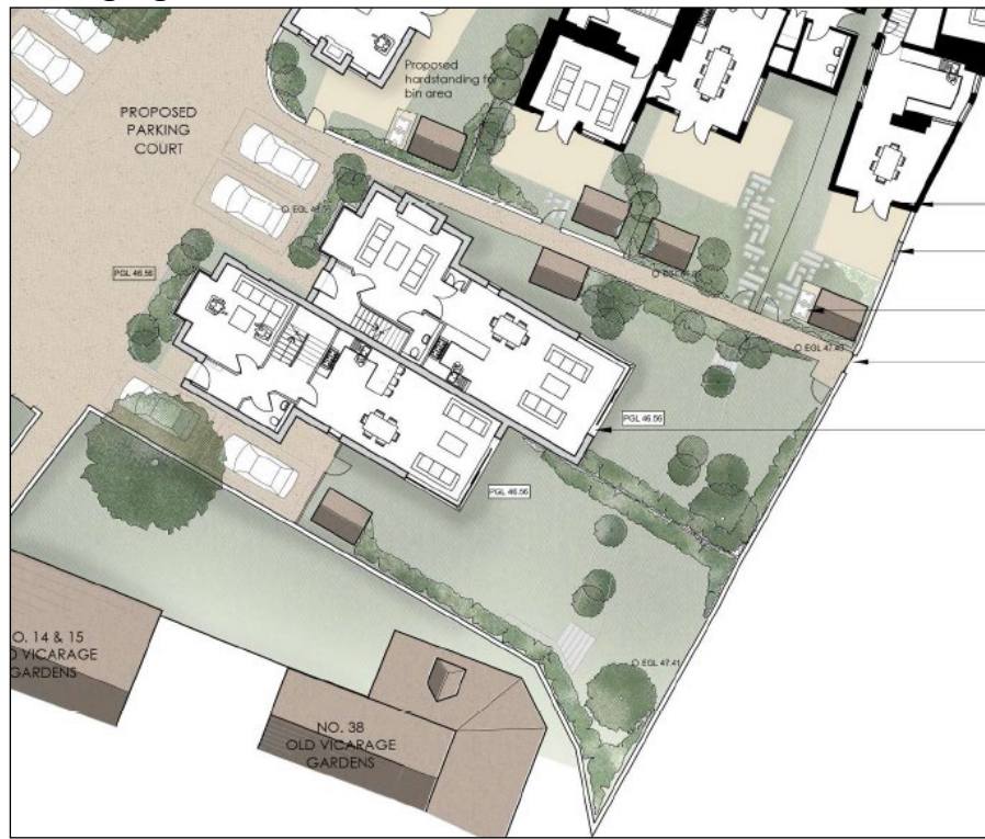
Figure 12 – The current proposal with unit 6 set forward and away from 16 Old Vicarage Gardens (incorrectly labelled on the plan as No.38) and in particular the rear dormer window.
