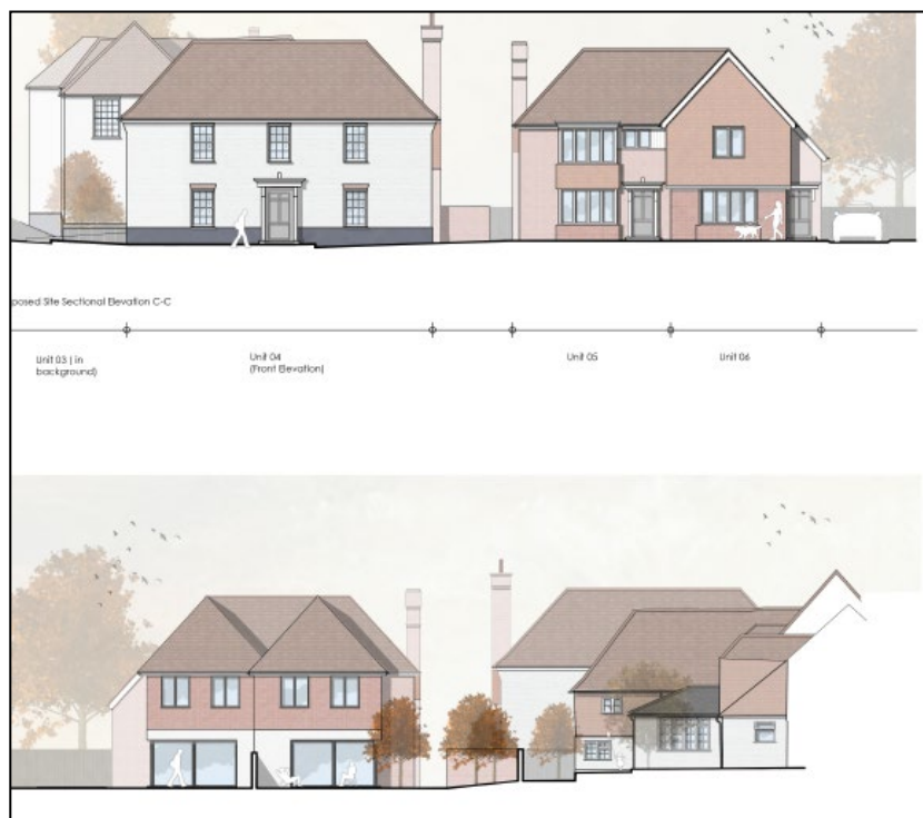
Figure 6: West elevation (above) showing ‘frontages’ of units 4, 5 and 6 and east elevation (below) showing rear of units 5 and 6.
